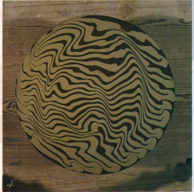
The beginning of the marbleizing process. The slab, resting on the bat, has been rotated or "joggled" to start the flow of the slips.
