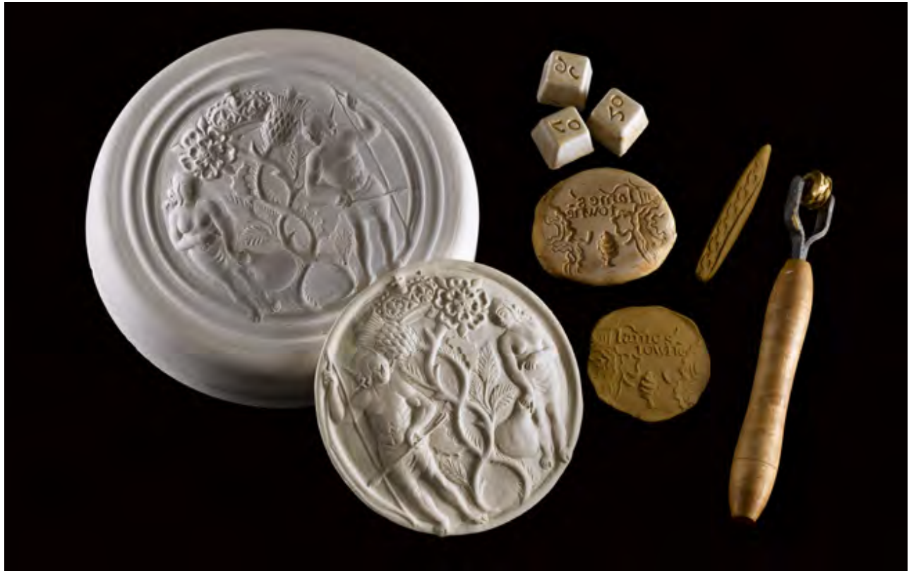
Figure 4 Maquette and related hand-carved spring molds and roulette wheel. D. of mold 8¼". (Courtesy, Michelle Erickson). This smaller prototype helped refined the larger medallion. Note the smaller molds for the dates and the “Jamestowne” lettering. The wood-handled brass roulette was used to emboss the rim of the medallion.
