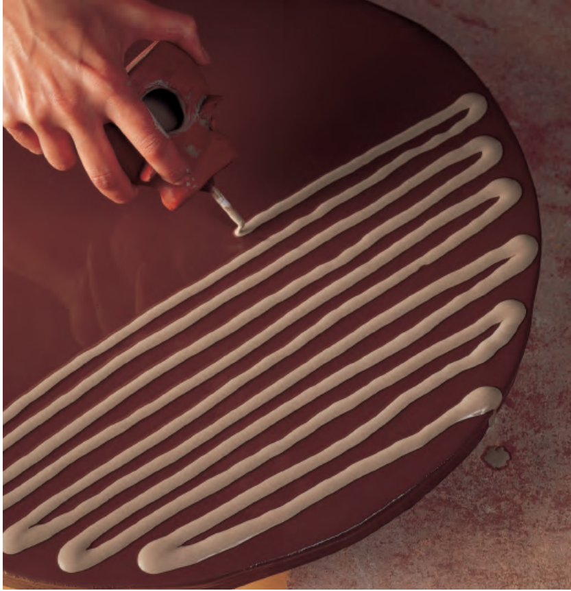
Figure 21 Parallel lines of white slip are immediately trailed onto the wet ground slip. The consistency and moisture content of the slips must allow both to flow easily without running. The width of the lines is dictated by the distance of the tip of the slip tube from the surface of the ground slip: the further from the surface, the wider the line.
