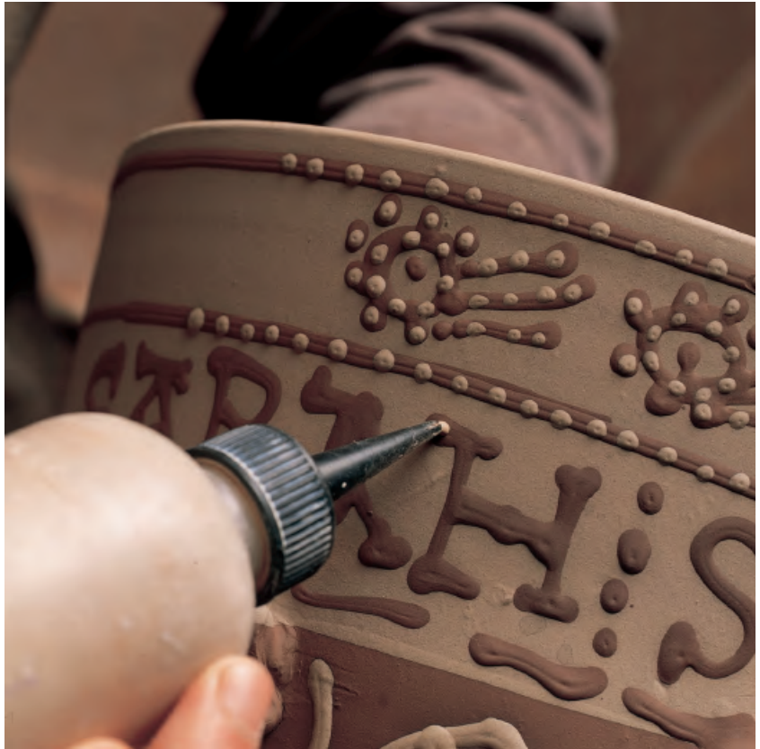
Figure 13 A final embellishment known as “jeweling” is applied. Small dots of white slip are used on top of slip lettering from the previously trailed black slip decoration.
