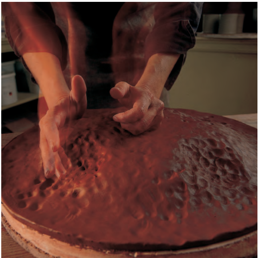
Figure 16 The depth of the carved relief requires that the slab be firmly pressed into the recesses. Slapping or pummeling the slab with a closed fist accomplishes this. After the dish firms up, it is removed and the edges are trimmed.
