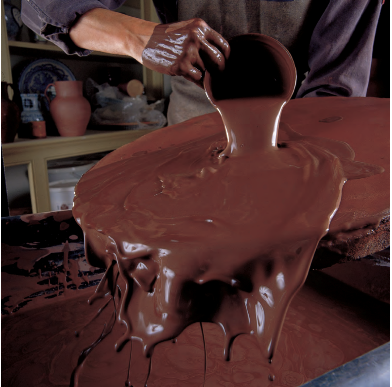
Figure 20 Creating a marbled-slip dish begins with a black ground slip poured over a flat , circular, red earthen clay slab, previously prepared and supported by a wooden bat. Slabs were prepared by rolling out the clay to an equal thickness.
