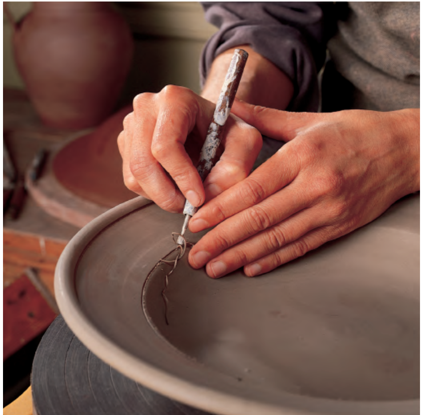
Figure 4 Once the slip covering has set up to a leather-hard stage, the sgraffito design is begun. The initial framing of the design is done on the wheel with the layout of concentric circles. The stylus is simply held in a fixed position while the wheel rotates, cutting the lines.
