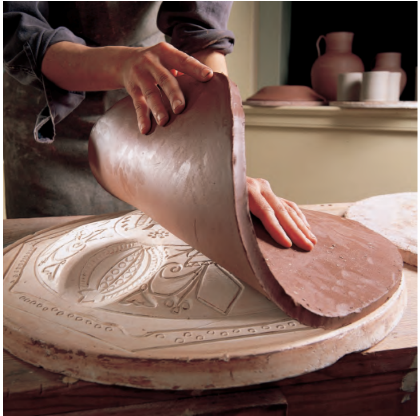
Figure 15 A circular clay slab is draped over a carved plaster mold. The clay is moist and very plastic at this stage. Period molds appear to have been made of fired clay.
