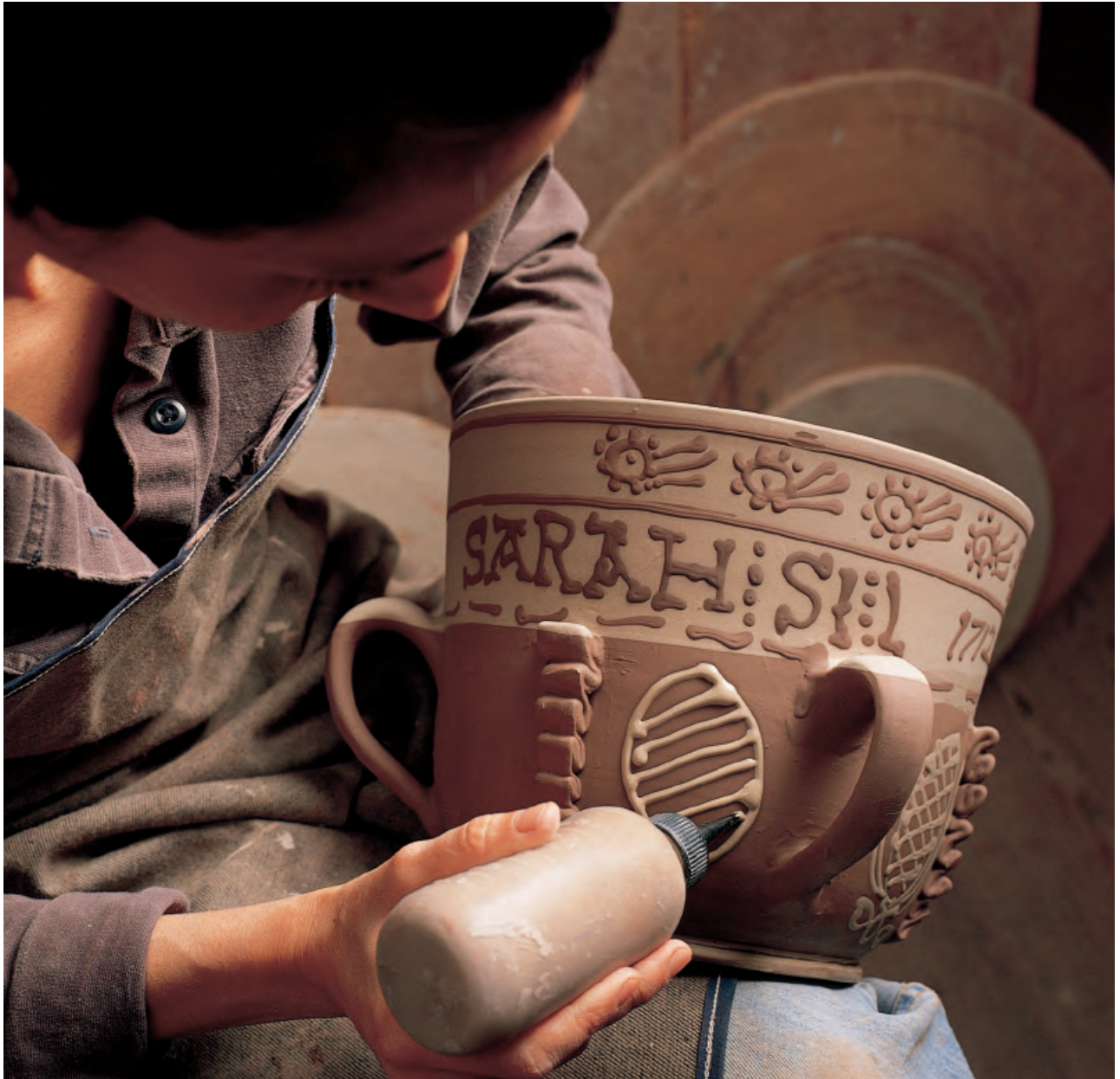
Figure 12 The initial layout of the design is started by applying concentric lines to the pot on the wheel. Black slip is used on the white ground slip where as a white slip is applied over the black ground slip. The decoration is done freehand and the vessel has to be turned carefully to avoid marring any of the previously applied trailing. A modern slip squeeze bottle is being used.
